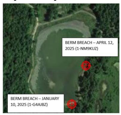
Figure 2: Cell 1 Lagoon Breach Locations
